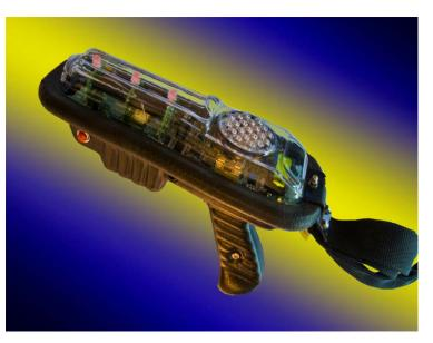
battery, front and rear triggers, and a grenade button. The electronics uses a switched-mode power supply for optimum battery life, and Surface Mount Technology for light weight and the highest possible electronic integrity
